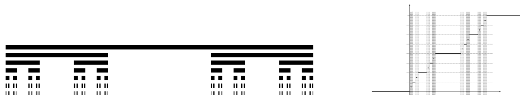
Seven stages of the construction of the Cantor set and graph of the Cantor function (from http://en.wikipedia.org/wiki/Cantor_set and http://en.wikipedia.org/wiki/Cantor_function )
